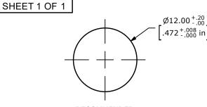
RECOMMENDED PANEL CUT-OUT 1-6mm THICKNESS
